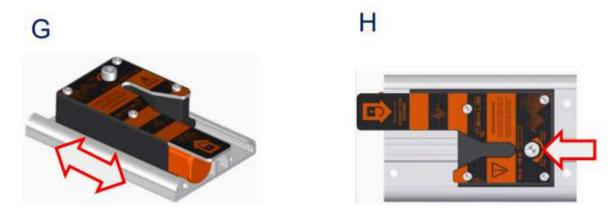
The stretcher safety lock must be installed in the position where the air wheel remains supported on the vehicle floor when removing the stretcher from the ambulance (I) (J) (K).
