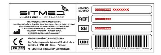
All Sitmed equipment is identified with a serial label for traceability control. The identification label is located on the bottom of the stretcher bed and contains the manufacturer's identification, product name, model, serial number, Anvisa (Brazilian Health Regulatory Agency) registration number of the Brazilian Ministry of Health, CE marking, and the Unique Device Identification (UDI-DI) number.
