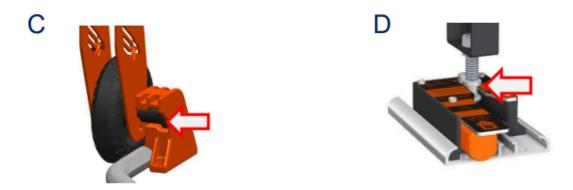
With the stretcher in the installation position, attach the front (C) and rear (D) anchoring system to the stretcher. The anchoring system must be adjusted with the minimum possible clearance to prevent oscillation during transport.
